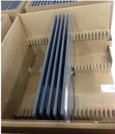
**Figure 4: Reusable paper separator to be placed between front faces of modules**
